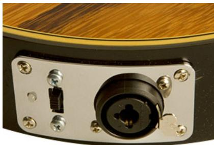
Plug the appropriate p into Dusk Tiger's output. For driving a standard amp, use a 1/4” stereo or mono guitar cable. For the LP-Z output, you will need either a custom length XLR male-to-XLR male cable, or use two standard XLR male-XLR-female mic cables in conjunction with an XLR male-to-male adapter (e.g. Radio Shack part #274-015). **Caution: When plugging the LP-Z output into a mic input, never turn on the input's phantom power. This may damage the Dusk Tiger output.**
