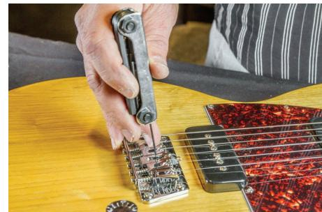
6. To Raise the Bender Saddle, loosen the 2 set screws a bit, loosen the hold-down screw by one turn – or enough to allow it to be raised to suit. Finally, snug the 2 set screws. Do not over tighten
