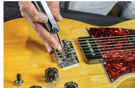
7. To lower the action, loosen the 2 set screws until the action is as desired, then snug the hold-down screw
